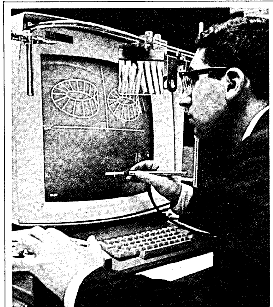
Three-dimensional pictures are being created by an IBM System/360 Model 50 computer at Brown University. Charles Strauss (above), a graduate student in the Division of Applied Mathematics, has programmed the computer to produce, on the screen of an IBM 2250 Display Unit, a pair of images that are similar but that differ slightly in perspective. As viewed through a stereoscope, the images merge into a single three-dimensional figure. The images can be enlarged, reduced, or rotated on the screen, and they can be altered by using a light pen.
